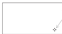
Cross marker Use the rotary knob <PICTURE> to move the marker. (The cross marker is half the length of the center marker and twice the width)
